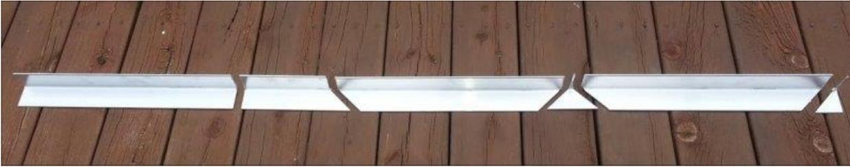
The 2" x 2" x 1/4" x 24" long angle is cut into 4 equal length sections with straight cuts. These are the 4 tower Feet, approximately 6" in length.
