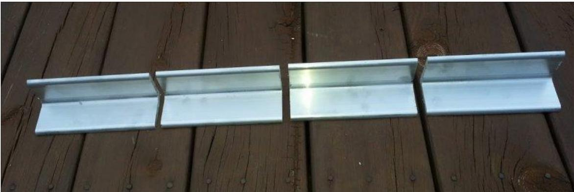
Each 1/8" x 2" x 48" flat piece is cut into 2 each 20" lengths with straight cuts, ending up with 8 each 1/8" x 2" x 20" flat pieces. These are the diagonal "X" braces. The corners of each piece may be cut at 45 degrees for a cleaner look.
