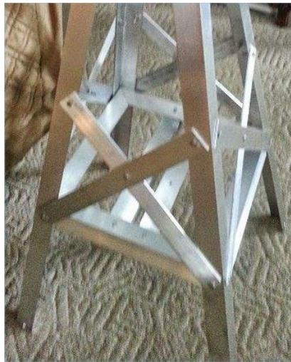
9. Attach the 2 rotor shelves to the lower shelf brackets with 4 each 5/16"-18 x 1" bolts and locknuts as shown above. Verify that all rotor mounting holes are 3.31" (Yaesu) or 3.0" (Hy-Gain) apart. Tighten these bolts securely. See the image at right above. These shelf brackets may fit tight.
